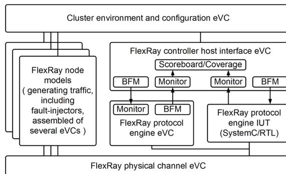
**Figure 1:** An overview of the NXP e VE, showing the PE-CHI interface in more detail
